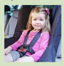
Forward facing combination child restraint with inbuilt six-point harness
